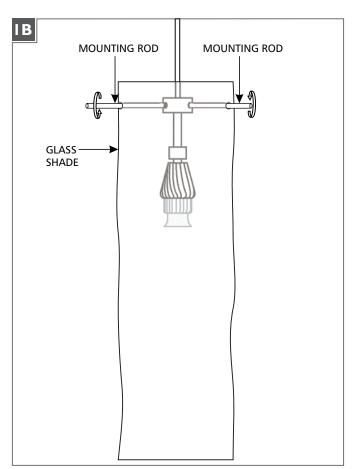
2 Place the hardware inside the glass shade and install the three mounting rods by screwing them in completely.
