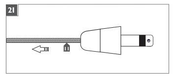
Pull the coaxial cable toward the fixture to smooth the wrinkles.
