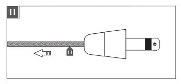
Pull the coaxial cable toward the fixture to smooth the wrinkles.
