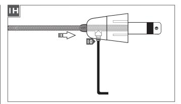
**IO** Firmly tighten the set screw on the conical connector.
