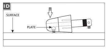
Tap the conical connector on a hard surface with the set screw facing down, so the plate inside drops into place.
