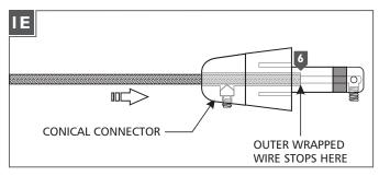
Feed and push the coaxial cable into the conical connector. The coaxial cable will come to a stop point after being inserted 3/4" into the conical connector.
