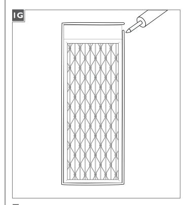
**I** For wet locations, caulk around the base with waterproof construction sealant.
