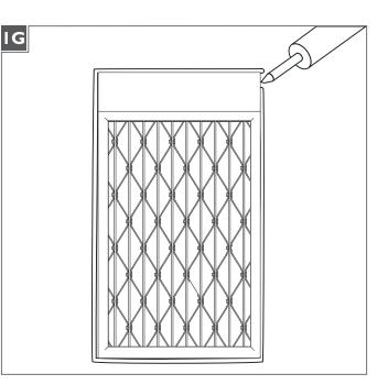
**I** For wet locations, caulk around the base with waterproof construction sealant.
