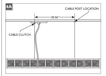
Mark the cable post location point 30.56" away from the center cable clutch on the canopy.
