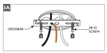
Mount the crossbar assembly to the electrical box with the two provided #8-32 screws.
