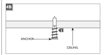
Tap the anchor at the marked point up to the threaded portion with a hammer.
