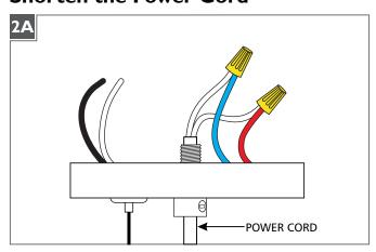
Take note of the wire connections and remove the wire nuts to disconnect the power cord wires from the driver wires.
