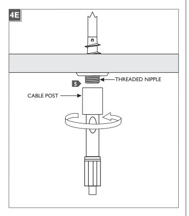
Screw the cable post completely to the threaded nipple.
