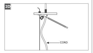
NOTE: The power cord does not support the fixture. For a casual "lazy cord" look, cut the power cord several inches longer that the drop height of the fixture.
