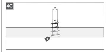
3 Screw the anchor in the rest of the way with a Phillips screwdriver.
