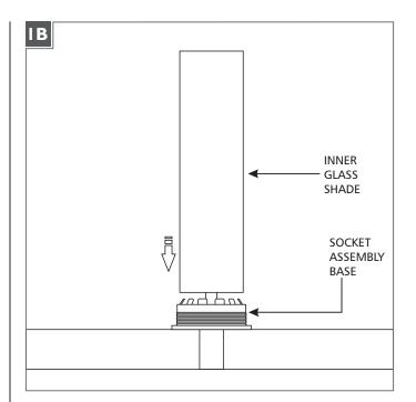
2 Gently push the inner glass shade into the center of the socket assembly base until it is firmly in place.
