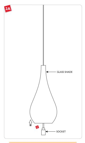
**NOTE:** To reduce the risk of a burn or electric shock during relamping, disconnect the power to the fixture.
