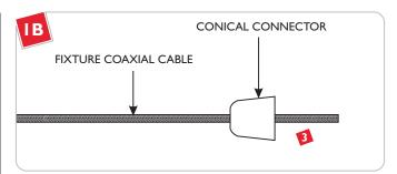
3 Insert the fixture coaxial cable through the conical connector.
