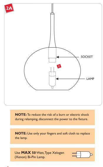
**1** Push the lamp pins completely into the socket holes.
