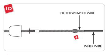
Slide the outer wrapped wire back to expose the inner wire.
