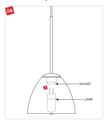
**NOTE:** To reduce the risk of a burn or electric shock during relamping, disconnect the power to the fixture.
