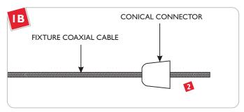
2 Insert the fixture coaxial cable through the conical connector.
