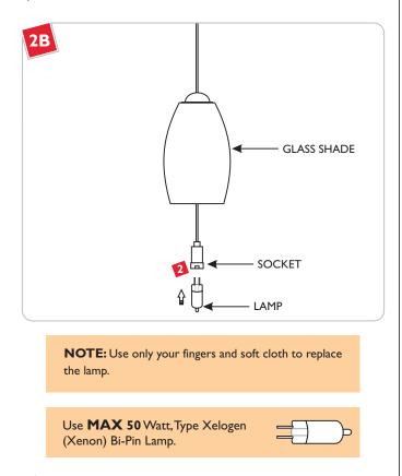
2 Push the lamp pins completely into the socket holes.
