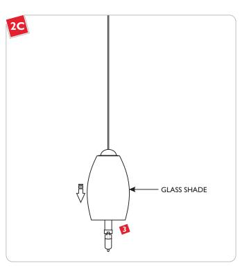
1 Lower the glass shade onto the socket assembly.
