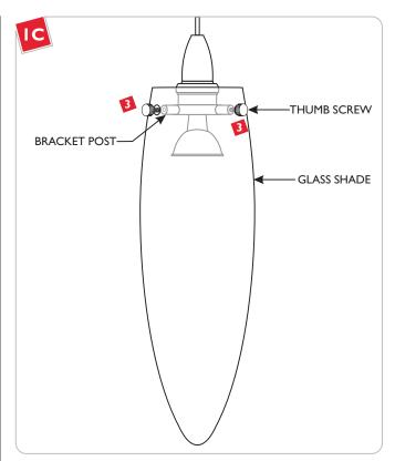
Place the glass shade completely into the bracket post and tighten the three thumb screws to secure the glass shade in place.
