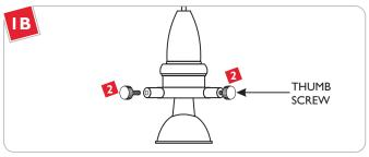
2 Remove the three thumb screws.
