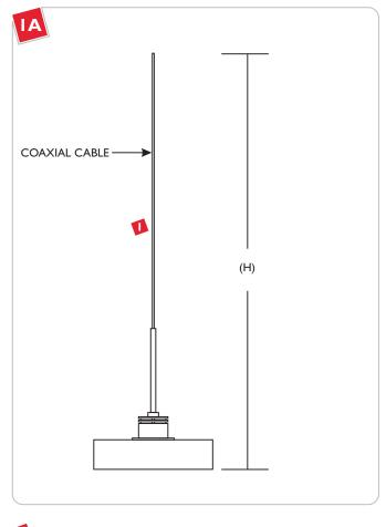
Cut the coaxial cable to the desired length with a sharp cutter. The overall fixture height (H) is measured from bottom of the metal shade to end of the coaxial cable.
