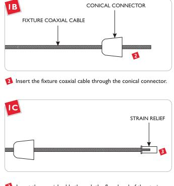
Insert the coaxial cable through the flared end of the strain relief.
