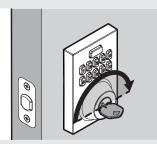
Close the door. Insert and rotate the key to lock the door. Ensure that the door locks smoothly.
