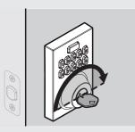
If your door does not lock and unlock smoothly, make sure you replaced your previous latch and strike with those supplied in the box. If you still experience locking errors, complete the troubleshooting steps at http://bit.ly/HC620jam or call Kwikset Support: 1-866-863-6584
