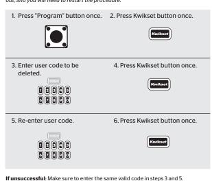
**Test code**: While the door is open, test the user code ake sure it no longer unlocks the door.
