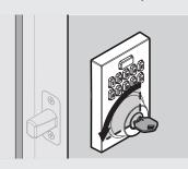
Turn the key 180° to retract the latch. Ensure that the door unlocks smoothly.
