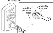
Fully insert your new key into the lock and turn it 180° counterclockwise. Next, turn the key 90° back to the starting position, then remove it.
