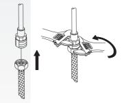
Apply pipe tape on threads of the inlet port. Tighten end of shank with wrench and slip hose into the inlet
