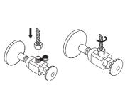
Apply pipe tape onto threads of the water supply. Tighten the hose onto water supply.
