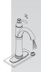
After installing faucet, remove aerator and turn on water to remove any left of debris. Re-assemble aerator.
