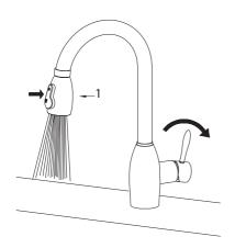
Turn the faucet on check if the spray head (1) switches modes properly by pressing the button
