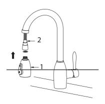
Screw the spray head (1) on the hose (2) and hand-tighten only
