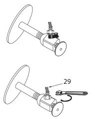
Screw hot & cold waterlines (29) onto the angle stops and tighten with an adjustable wrench until snug
