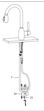
Install the weight (24) at the lowest point (horizontally) on the hose (2) and tighten the screws (25) with a Phillips head screwdriver
