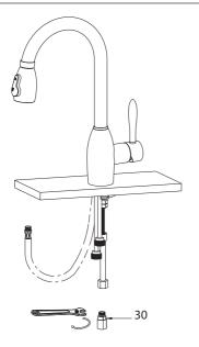
Screw the check valve assembly (30) onto the mounting pipe.
