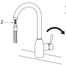
Turn the faucet on while holding the tip of the hose (2) to flush any debris
