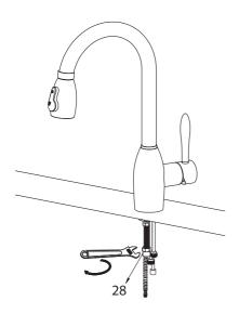
Place the plastic nut (28) on the mounting pipe and tighten with an adjustable wrench (not included) until snug (Note: The plastic nut only tightens at the end of the mounting pipe)
