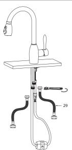
Connect hot & cold waterlines (29) onto the faucet hot and cold inlets (hot: long & cold: short), and tighten with an adjustable wrench until snug
