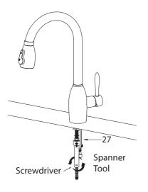
Tighten the metal nut (27) on the mounting pipe with the provided spanner until snug underneath the countertop. Installer Tip:
