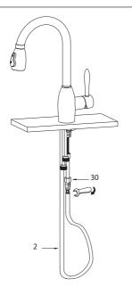
Screw the end of the hose (2) onto the check valve assembly (30) and tighten with an adjustable wrench until snug
