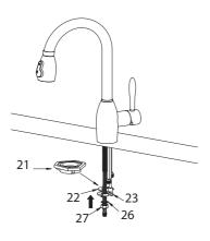
Install the faucet extender (21), rubber u-washer (22), and metal u-washer (23) on the mounting pipe until it touches the base of the countertop. Place metal o-ring (26) and screw metal nut (27) onto the mounting pipe
