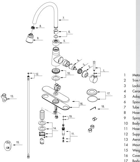
Metal Handle Assembly Trim Cap Locking Nut Ceramic Disc Cartridge Adapter Spout Seal Kit Tube Assembly Hose Guide Spray Head Body Trim Ring Hose Adaptor Assembly Supply Hose Aerator Wrench Mounting Hardware Assembly Weight Cover Plate& Putty Plate Body Trim Ring Hex Wrench (H2.5 \* 19 mm L \* 53 mm L) 18 O-Ring set(Φ1/4" ID \* Φ3/8" OD) 19
