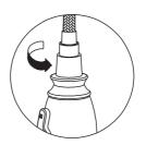
Note: Check if O-ring is visible in the hose (2) prior to reinstalling the spray head (1)
