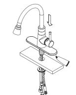
Place silicone sealant beneath the bottom plate and install faucet through center
