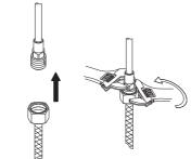
Tighten end of shank with wrench and slip hose into the inlet port.
