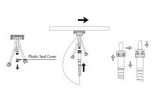
Remove the plastic seal cover from the outlet port prior to pushing the hose adapter onto the same port, you will hear a "click" sound once they are
