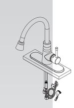
Attach metal weight to the hose to prevent hose from twisting. Return hose to proper
