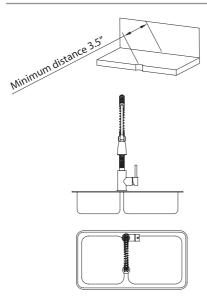
The minimum distance between the faucet hole and the wall should be 3.5"
