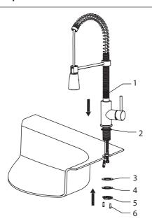
Insert the faucet body (1) into the hole on the deck with the base o-ring (2). Install the rubber washer (3), metal washer (4), mounting nut (5) and mounting screws (6) from underneath the sink
