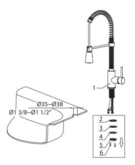
Remove mounting screws (6), mounting nut (5), metal washer (4), and rubber washer (3) from the faucet body (1)
