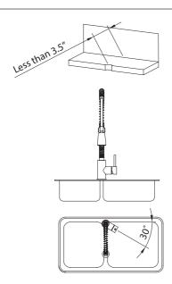
If the distance between the faucet hole and the wall is less than 3.5", position the faucet lever 30 degrees to 90 degrees off of the wall to allow for full operation
