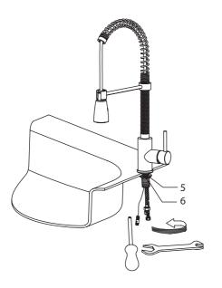
After adjusting the direction of the faucet body (1), tighten the mounting nut (5) until snug and tighten the mounting screws (6) to the nut with a Philips head screwdriver
