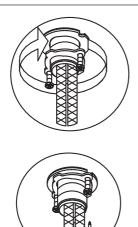
Adjust direction of faucet body (5). Tighten mounting nut (6C) until snug. Tighten mounting screws (6D) to nut with a Phillips head screwdriver until snug
