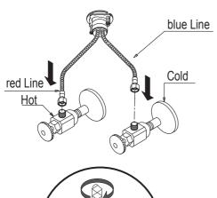
Connect hot and cold waterlines (7) to the angle stops. Tighten with a wrench until snug. Turn on hot and cold angle stops and check for leaks
