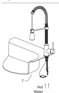
Connect the spray hose (9) to the supply line and tighten with a wrench until snug, then install the weight (7) at the lowest point (horizontally) on the spray hose (12)
