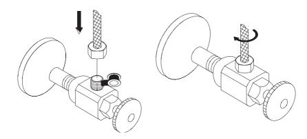
Connect hot and cold waterlines (12) to the angle stops and tighten with a wrench until snug, then unscrew spray head (8), hold the tip of the spray hose (9) and turn on the faucet to flush any debris
