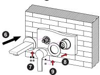
Install connecting pole 15 to the spout 10. Screw the set screw 12 into spout 10 with alley key and install the decorative cap 11. Install handle 8 to the corresponding position to valve 17. Tighten decorative screw 6 with alley key and place cap 7 afterwards.
