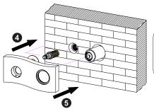
Place sufficient Teflon tape on connecting pole 15. Screw it into corresponding screwed hole of valve 17 (If the connecting pole is too long please shorten it with a saw; refer to dimensions for detail size). Install decorative board 13 and Fixing board 14 to valve.
