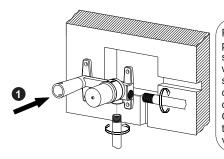
Place sufficient Teflon tape on hot/cold water supply pipe lines. Insert them into the corresponding threaded screw of valve 17 and install it into the wall. Open the water supply to check if there is leakage. Loosen screw 3 and take the plastic cover 2 off. Open the cartridge to make sure there is no leakage. Close the cartridge after checking. Remove plastic cover 16. Open cartridge and remove the dirt in the pipe. Close the cartridge and install the plastic cover 16 and 2 into valve.
