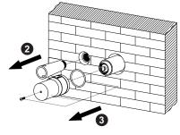
Seal the wall after checking for leakage. If there is no leakage, remove plastic cover 16 and 2.
