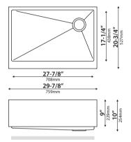
\* KHF410-30 29-7/8" x 20-3/4" x 10" Min Cabinet Size: 33" Matching Grid: KBG-410-30 Drain Model #: ST-1 Drain Cap: STC-2
