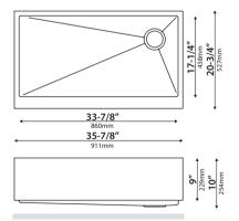
\* KHF410-36 35-7/8" x 20-3/4" x 10" Min Cabinet Size: 39" Matching Grid: KBG-410-36 Drain Model #: ST-1 Drain Cap: STC-2
