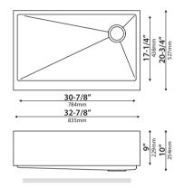
KHF410-33 32-7/8" x 20-3/4" x 10" Min Cabinet Size: 36" Matching Grid: KBG-410-33 Drain Model #: ST-1 Drain Cap: STC-2
