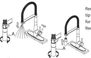
Remove spray head (A). Hold tip of spray hose. Turn faucet on for 1 minute to flush any debris. Reconnect spray head (A)
