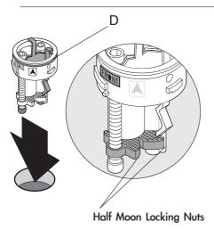
Insert base (D) into sink or countertop with "FR↑NT" facing forward. Tighten screws on base (D) with 4mm hex wrench (F) until base is secure on sink or countertop
