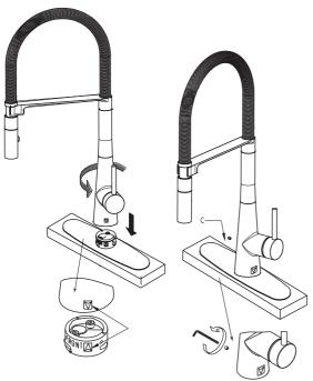
Align arrow on faucet body (B) with arrow on base (D). Attach faucet body (B) to base (D) and turn counter-clockwise. Secure faucet body (B) by tightening the set screw with 2.5mm hex wrench (J)
