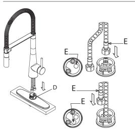
Insert hot & cold waterlines (E), one by one, in large hole of base
