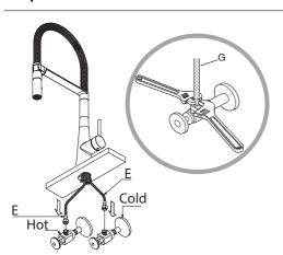
Thread hot & cold waterlines (E) onto angle stops. Tighten with adjustable wrench until snug. Turn on the angle stops and check for leaks (DO NOT TURN FAUCET ON)
