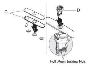
Place a bead of clear silicone sealant (not included) around the edge of the putty plate (C). Secure deck & putty plate (C) on sink or countertop. Insert base (D) into hole of deck & putty plate (C) with "FR↑NT" facing forward. Tighten screws on base (D) with 4mm hex wrench (F) until base is secure on deck & putty plate (C)
