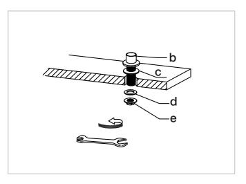
Screw the dispenser bottle (f) to the dispenser base (b) from underneath the countertop. Tighten as required. Fill the dispenser bottle (f) from the top with 12 ounces of soap
