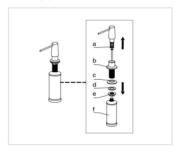
Install dispenser base (b) with rubber washer A (c) attached into the hole in the countertop. Re-install rubber washer B (d) and mounting nut (e) on the dispenser base (b) from underneath the countertop. Tighten mounting nut (e) with adjustable wrench until snug
