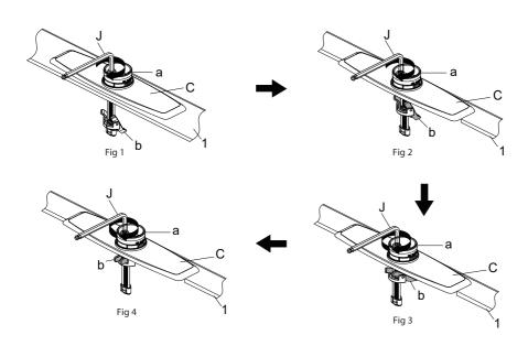
Press the base (a) and escutcheon (C) so that they can not move, then turn the screws with the provided hex wrench (J, HEX: 6.0mm) clockwise, as shown Fig 1. When the mounting plates (b) make contact with the sink (1), continue to turn the screw with the provided hex wrench (J, HEX: 6.0mm) clockwise, as shown Fig 2, until the base (a) is completely tightened and secured, as shown Fig.4.
