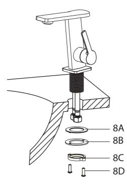
Install faucet through 1-3/8" predrilled hole in countertop. Attach rubber washer (8A), metal washer (8B), mounting nut (8C), and mounting screws (8D) on the threaded mounting pipe. Tighten mounting nut (8C) until snug. Tighten screws (8D) on mounting nut (8C) with Phillips head screwdriver until snug
