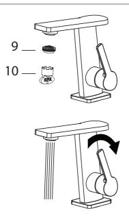
After installing faucet, remove aerator (9) with included aerator key (10). Turn water on for 30 seconds to remove any debris. Reassemble aerator (9)
