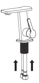
Place faucet on a soft cloth, spout facing up. Attach the waterlines into the base of the faucet (HAND-TIGHTEN ONLY) (A)Hot side left (B)Cold side right
