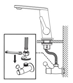
Connect flex water supply lines to angle stops and tighten with adjustable wrench. Turn on both hot and cold main valve
