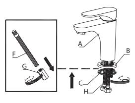
Remove faucet, mounting hardware, and waterlines from the box. Remove mounting nuts (G) from mounting screws (F). Place faucet body (A) on a soft cloth, spout facing up. Secure hot & cold waterlines (H) at the base of the faucet (HAND-TIGHTEN ONLY)
