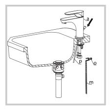
• Insert lift pole rod (p) through the hole in the back of the faucet body (a). Loosen thumb screw (o) and attach extender rod (m) to lift pole rod (p). Tighten thumb screw (o)
