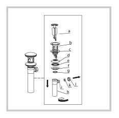
• Remove waste stopper (a) from drain (b). Remove tail pipe (h), mounting nut (f), plastic washer (e), and concave washer (d) from drain (b). Remove retaining nut (l) and washer (k) from tailpipe (h)
