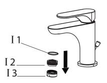
Remove aerator assembly (I). Loosen aerator cover (I 3) with adjustable wrench. Remove aerator (I 2) and aerator washer (I 1). Turn water on for 1 minute to remove any debris. Reassemble aerator assembly (I)
