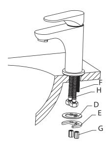
Install rubber O-washer (D) and metal U-washer (E), over waterlines (H) and mounting screws (F), from underneath the countertop or sink. Attach mounting nuts (G) to mounting screws (F) and tighten with adjustable wrench or 10mm wrench until snug
