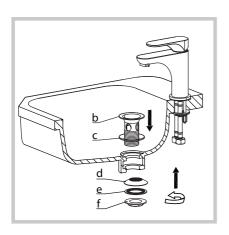
• Install drain (b), with rubber washer (c) attached, into the drain hole. Attach concave washer (d) with narrow end up, plastic washer (e), and mounting nut (f) to drain (b) from underneath countertop or sink. Secure tightly to sink with an adjustable wrench
