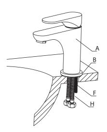
Install faucet body (A) through 1-3/8" hole in countertop or sink, with hot & cold waterlines (H), mounting screws (F), and base metal ring (B) attached
