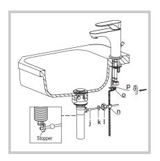
• Insert shortest end of drain off pole (j) into drain off pole opening of tailpipe (h). Make sure drain off pole (j) and slot on waste stopper (a) engage. Attach washer (k) and retaining nut (l) through drain off pole (j). Secure retaining nut (l) to drain off pole opening of tailpipe (h)
