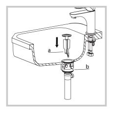
• Insert waste stopper (a) into drain (b). Make sure slot at end of waste stopper (a) is facing the rear of the sink
