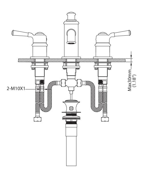
Step1: Remove mounting hardware and three-way connector
