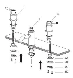
Install faucet body (2), hot handle valve (1), and cold handle valve (3) through 1-3/8" predrilled hole in countertop. Attach rubber washer (5A), metal washer (5B), mounting nut (5C), and mounting screws (5D) on the threaded mounting pipe. Tighten mounting nut (5C) until snug. Tighten screws (5D) on mounting nut (5C) with Phillips head screwdriver until snug. Attach three-way connector (7) to faucet body (2)
