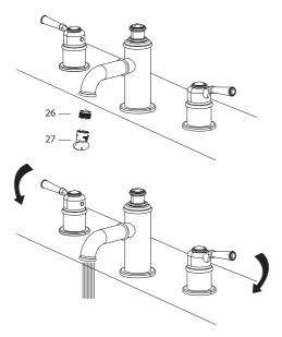
After installing faucet, remove aerator (26) with included aerator key (27). Turn water on for 30 seconds to remove any debris. Reassemble aerator (26)
