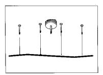
**Step 4.** While supporting the rail, screw the transformer power feed cap back onto the transformer. The connection must be tight.
