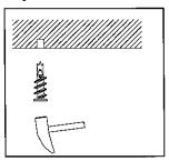
**Step 7.** Finish the installation using a screw driver to screw the anchor until is flush to the ceiling.
