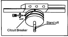
2. Transformer is equipped with a circuit breaker. It is located on the side of the upper setcion of the transformer. This will "trip" (turn off power) if too many fixtures are put on the track or there is a short circuit. To reset circuit breaker push button in. If it continues to trip make sure that the total wattage of all fixture does not exceed 60 watts. Also make sure there is no conducting material shorting out the track.
