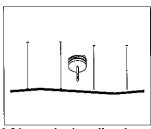
**Step 6.** Line up the drywall anchors with the marks on the ceiling and use a hammer to tap the anchor approximatelly 1/2" into the ceiling. Stop just before the threaded portion of threaded portion of the anchor enters the ceiling.
