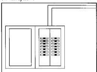
Step 2. Turn on the light system and let it run for 5 minutes. Turn the system off, carefully check that all connection points are not hot to the touch (warm is acceptable), if a connection is hot, check the connection and make sure the wire nut is tightly secured.
