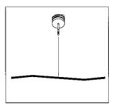
Step 3. The transformer and the standoffs will be used to support the rail from the ceiling providing a total of five supports. Use a pencil and tape measure to mark two of the support locations on the rail 6" from each end of the rail.
