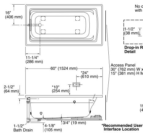
No change in measurements if connected with drain illustrated. (K-7272)
