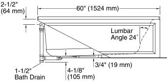
No change in measurements if connected with drain illustrated. (K-7272)
