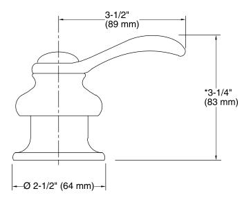
\* Allows for +/- 1/4" (6 mm) handle adjustment.
