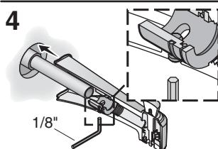
Loosen the setscrew and slide the spout against the wall.
