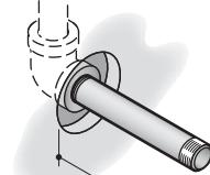
The nipple should extend 4-1/8" (10.5 cm) past the finished wall.
