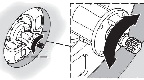
**11** Reinstall the collar with the setscrew against the tab.
