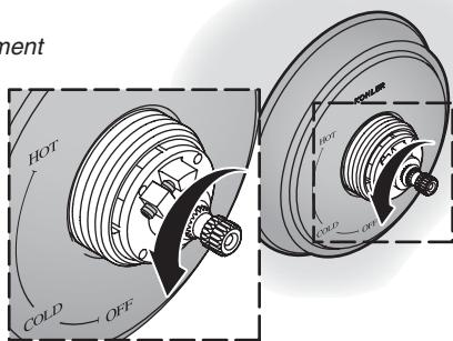
**23** Attach the stem adapter. Begin with the standard wall installation. Attach the handle. If the stem adapter is too long or the handle bonnet is not tight against the escutcheon, turn the stem adapter around and try the shallow wall installation.
