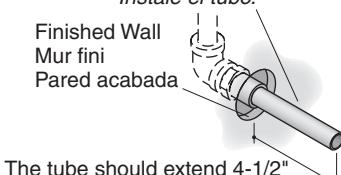
The tube should extend 4-1/2" (11.4 cm) - 5" (12.7 cm) past the finished wall.
