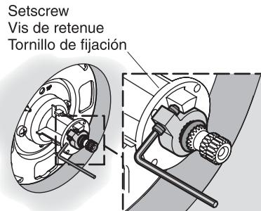
For minor temperature changes, adjust the setscrew and recheck the temperature.
