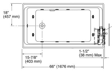
No change in measurements if connected with drain illustrated. (K-7147-AF)
