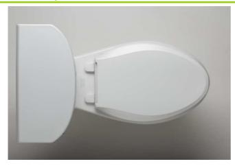
Toilet shall be 28-3/4" (730 mm) in length, 17-5/8" (448 mm) in width, and 30-3/4" (781 mm) in height. Toilet shall be made of vitreous china. Toilet shall be 1.28 gpf (4.8 lpf). Toilet shall feature touchless actuation. Toilet shall be Comfort Height®. Toilet shall be a 12" (305 mm) rough-in.
