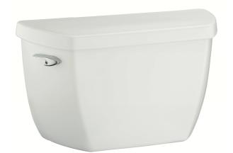
The tank shall be made of vitreous china. Tank shall be 8-5/8" (219 mm) in length, 21-1/4" (540 mm) in width, and 14-1/4" (362 mm) in height. Tank shall be 1.0 gpf (3.8 lpf). Toilet shall be equipped with Sloan FLUSHMATE® - Sloan® Valve Company. Toilet shall include a polished chrome trip lever.
