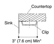
\*Allow clearance around the back sink rim for clip attachment.
