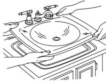
Immediately wipe away any excess sealant, and fill any voids as needed.
