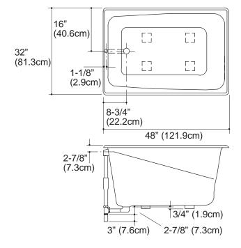
No change in measurements if connected with drain illustrated. 46-1/2" (118.1cm) x 30-1/2" (77.5cm) Cut-out
