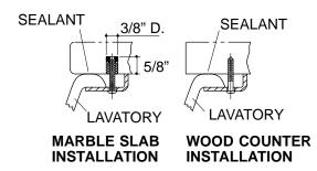
NOTE: WATERPROOF UNPROTECTED OVERHANG AREA ON THE UNDERSIDE OF WOOD COUNTER.
