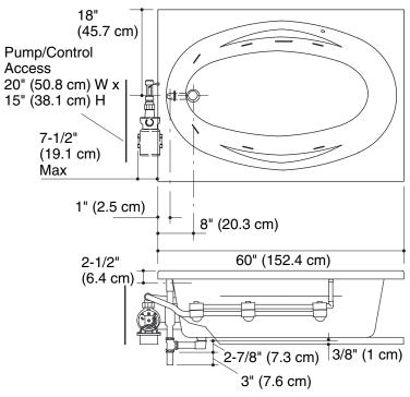
No change in measurements if connected with drain illustrated. (K-11677)
