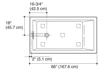
No change in measurements if connected with required drain illustrated. (K-7272)
