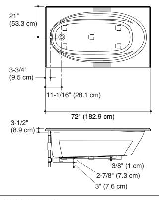
No change in measurements if connected with drain illustrated. (K-11677 or K-11677M)
