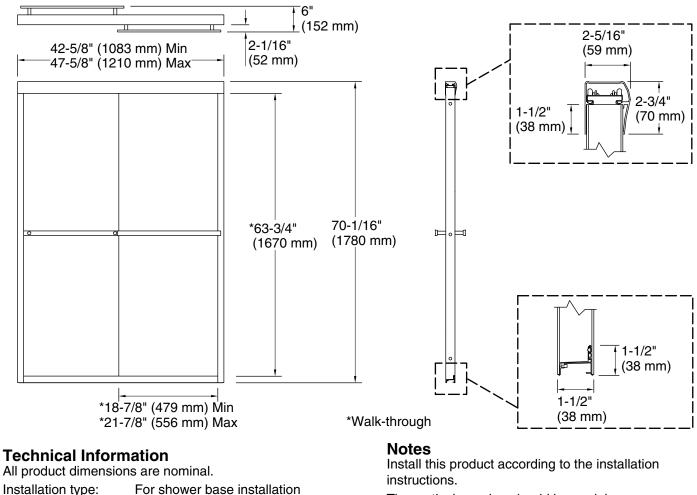
The vertical opening should be a minimum of 72" (1829 mm) to allow for installation clearance.
