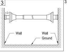
Holding the larger sized rod, rotate the smaller rod until it is locked into position securely.
