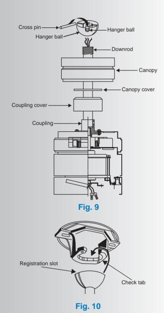
Step 8. Slip the coupling cover, canopy cover and canopy onto the downrod.
