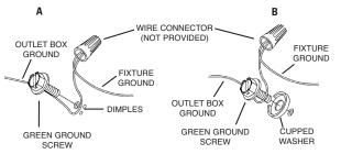
Make wire connections (connectors not provided.) Reference chart below 5) for correct connections and wire accordingly.
