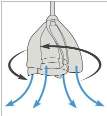
Terna<sup>™</sup>'s contoured blade design produces a unique outward airflow pattern to cool a wider area.
