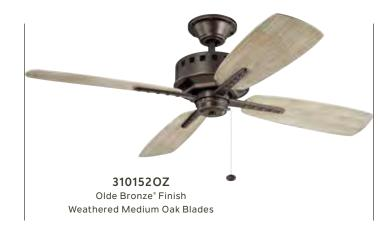
Blades (4) Included - 14° Pitch - 52" Sweep - Non-reversible - ABS **Downrods** 4.5" Downrod with 1" (O.D.) Downlight N/A Downlight Glass N/A Optional Downlight See pages 318-320 Uplight N/A Uplight Glass N/A Low Ceiling Adaptable No **Control** Pull Chain
