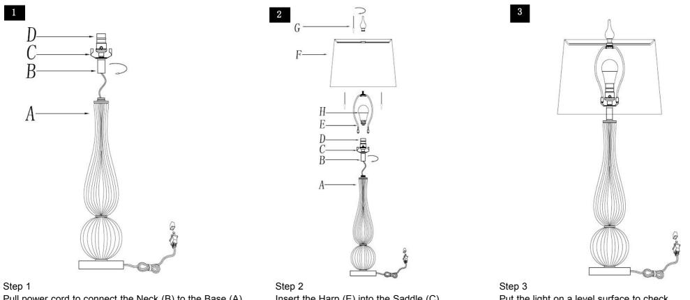
Pull power cord to connect the Neck (B) to the Base (A). Screw the Neck (B) onto the Lamp base (A) Be careful not to twist the power cord and tighten securely
